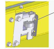
Make sure that the extension deck is in locked position.
