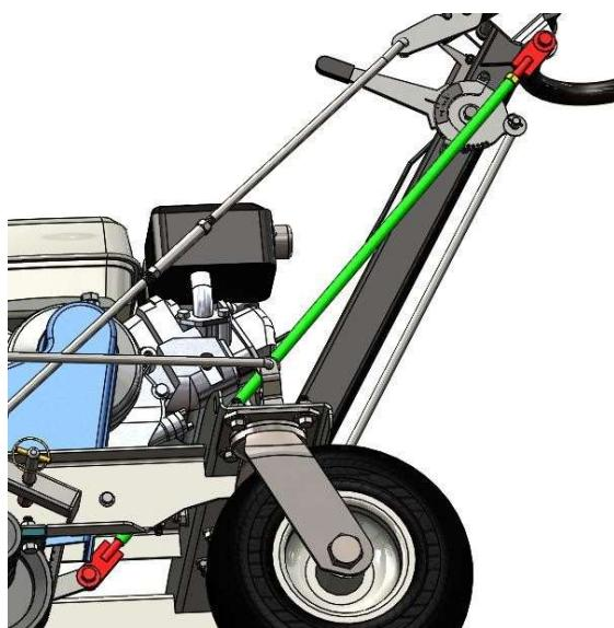
1. Loosen the (yellow) jam nut to release the tension.
