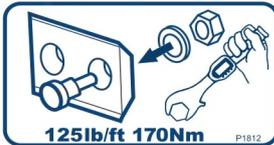
P1812 | Torque blade bolts to 125 lbs ft (170 Nm).                                                                                                             |                                                                                              |
