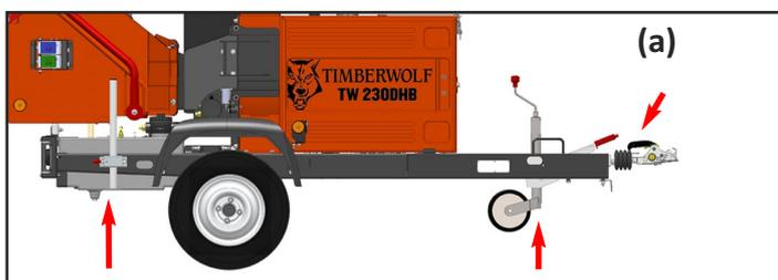
When the chipper is unhitched it should be level and made secure before starting work by applying the handbrake and lowering the prop stand and jockey wheel (b).
