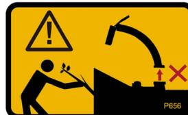
P656    | Danger.<br>Do not use this machine without the discharge unit fitted. Failure to comply may result in serious injury or damage.                        |                                                                                              |
