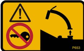
P653    | Danger.<br>Rotating blades inside.<br>Stop engine and remove key before removing discharge unit.                                                       |                                                                                              |
