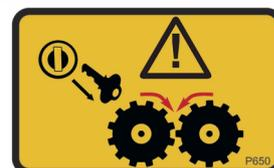
P650    | Danger.<br>Autofeed system fitted. Rollers may turn without warning! When the engine is switched off the rollers will turn during the run down period. |                                                                                              |
